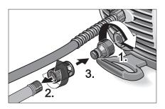
**Step 3**Connect garden hose to unit's water inlet using the quick connect adapter.
